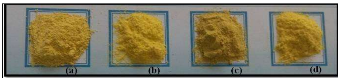
Figure1. Colors of (a) LiNiPO 4 , (b) LiNiPO 4 doped carbon, (c) LiNiPO 4 doped carbon and silver and (d) LiNiPO 4 doped carbon and Aluminum powders.
