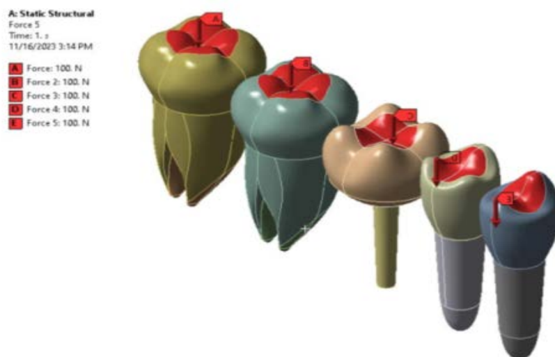
Figure 4: An applied vertical occlusal load of the implant.
